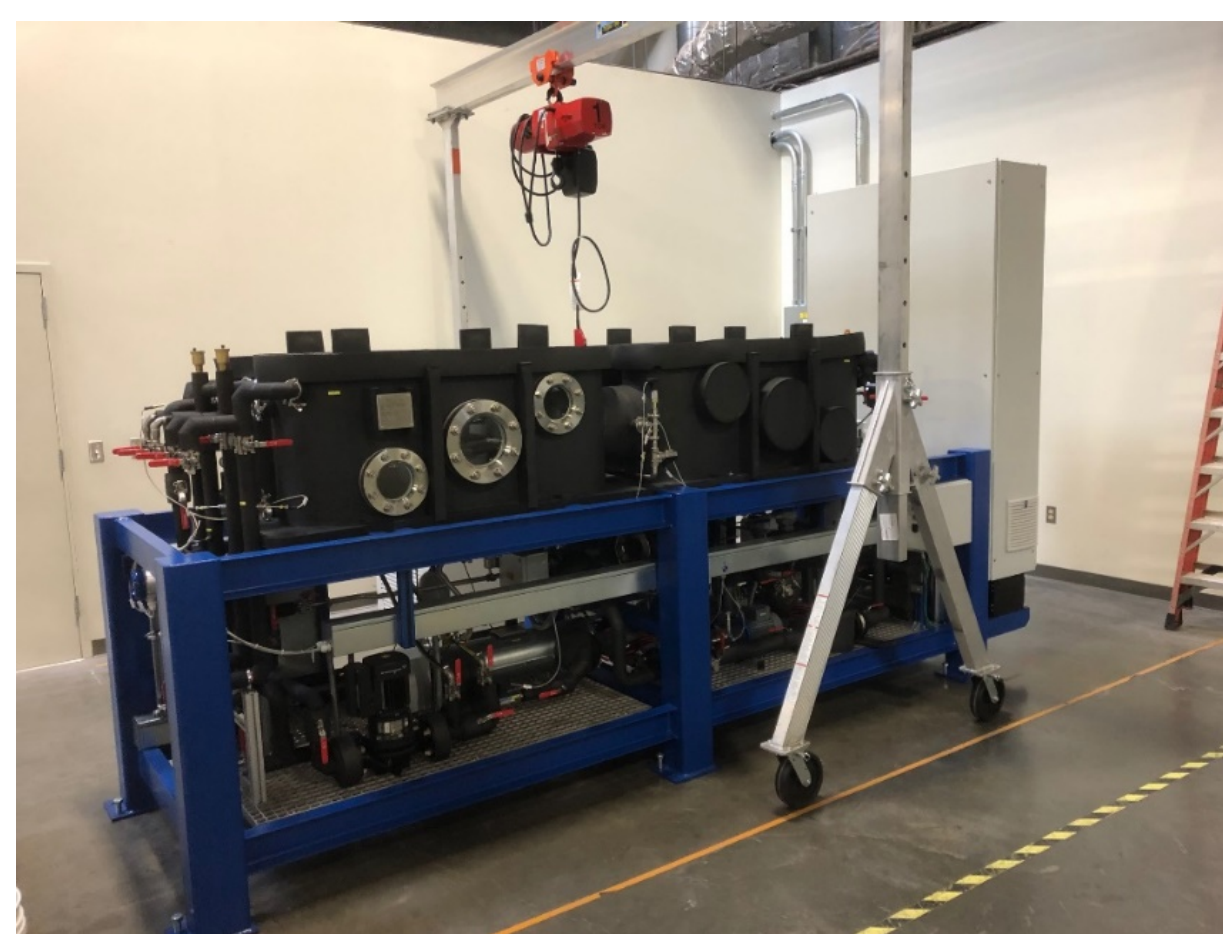
An absorption chiller test-rig was custom-designed and built to investigate novel working pairs
